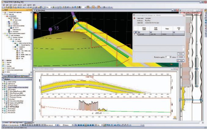
The Drilling Visualization plug-in allows users to create extrapolations from deviation surveys, predict upcoming events, estimate expected formation depths, monitor changes to model data, provide audible notifications, and run workflows. Bottomhole assembly and bit positions can be viewed in the context of Earth, improving the understanding of current operations and identification of drilling events.
