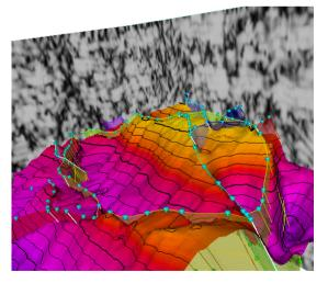
Figure 2: Surface with fault model and seismic data
